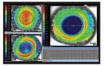
Fully Automatic image capture makes patient testing simple and quick. Simply position the instrument, guided by the intuitive 3D focusing target, and the software does the rest. Each video frame is analysed for centering, focus and movement. The best four frames are automatically captured and displayed in the image windows above.
